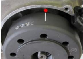
Place the rotor loosely onto the crank and check that it may move freely above the statorbase.
