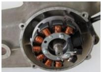
Magnet based generator with integrated solid state ignition. Light output 12V/70W AC. Ignition with own power supply from within the system. Replaces original Magneto as well as all ignition parts. Does not require changes on crankcase.
