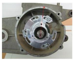
Now transfer the timing mark on the engine housing of the stator base. Extend to the imaginary line from the center of the crankshaft timing mark on the addition.
