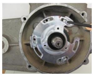
Remove the 3 screws that hold the new stator on its base and pull it away from the plate. Be careful not to damage the paint insulation of the coil wires.
