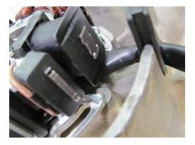
**Ignition timing:** To get maximum flexibility no groove has been put into the rotor. No need to worry over the now lost woodruff key. It did not have an arresting capacity, it was guiding to correct ignition settings. Now you have the markings and a much greater flexibility.
