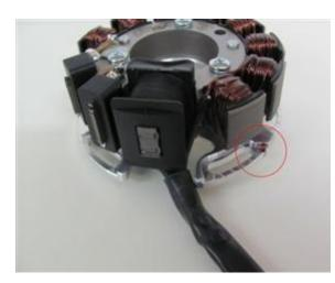
Explore the base plates. When you see a red cable exit point as a timing mark. Since this is no longer visible when attached rotor, you must later be transferred to the motor housing.
