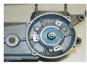
Unscrew the old stator and take it off the engine. Pull the rotor off, you will need a puller for this. Take the woodruff key from the crank. You will not need it anymore. Please do not forget to do so, otherwise you will have trouble later on in the assembly. (Remark: This woodruff key does not actually hold your rotor on the shaft, this is done by the cone. It simply guides to the correct setting which will now be otherwise achieved.)
