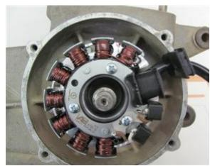
Put the stator coil to the support plate. Make sure that the cable and the thick black coil pointing in the direction of the cable output of the engine.
