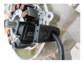
The cable from the stator there is a grommet. These can be attached to the housing. This spout maintains the cable and preventing it from dragging on the rotor.
