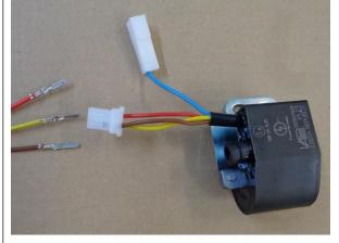
... Take the female connector of the ignition coil with the cable colours yellow, red and brown.
