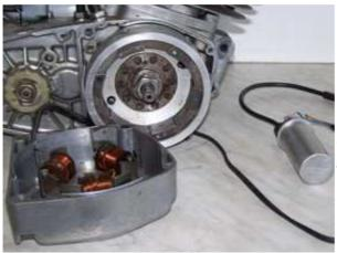
Disconnect all wires of the old magneto and the ignition coil and remove those parts. If you have any additional adapters installed for alternatively generators - please remove them too.
