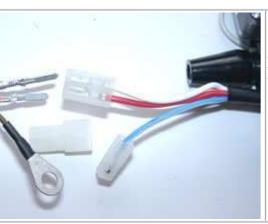
Look for the ignition coil with its female plug and the two wires (red and white).
