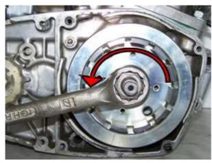
Now place the new rotor onto the crank shaft (as shown in the picture).
