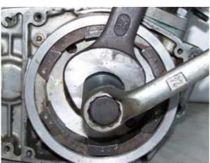
Next, pull the stock rotor from the crank shaft by using a puller tool (presumably M36x1,5 -Not provided!-)
