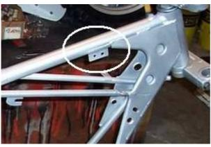
Fasten the new ignition coil there, say where the original coil had been sitting (or any other convenient place). Note that there will have to be a ground wire attached during wiring. Screw the ht-cable into the coil. Secure the new wiring to the frame.
