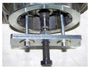
The new rotor should **ONLY** be removed with the supplied puller (part-no.: 72 09 799 99).
