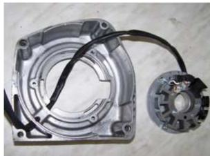
Pull the wiring of the stator through the cable exit of the engine cover. Do this very carefully - it is very tight. Better give it some greasing at the insulation of the wiring harness.
