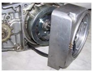
Now lead the harness carefully through the engine's cable exit. Again, a tight thing, so watch out not to damage the insulation.
