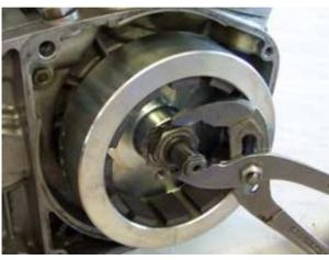
Make sure that the securing washer with external tab is neatly folded around the nut so that nothing of its perimeter reaches beyond the perimeter of the nut.
