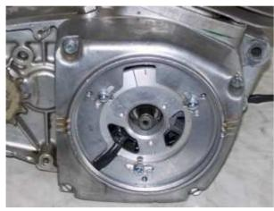
Place the dynamo cover (with the assembled stator unit) onto the engine. You will help the cable by gently pulling on it from the other side (though the engine).
