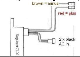
The new regulator/rectifier has 4 wires
