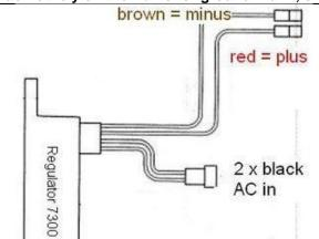
The new regulator/rectifier has 4 wires
