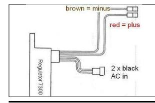
The new regulator/rectifier has 4 wires
